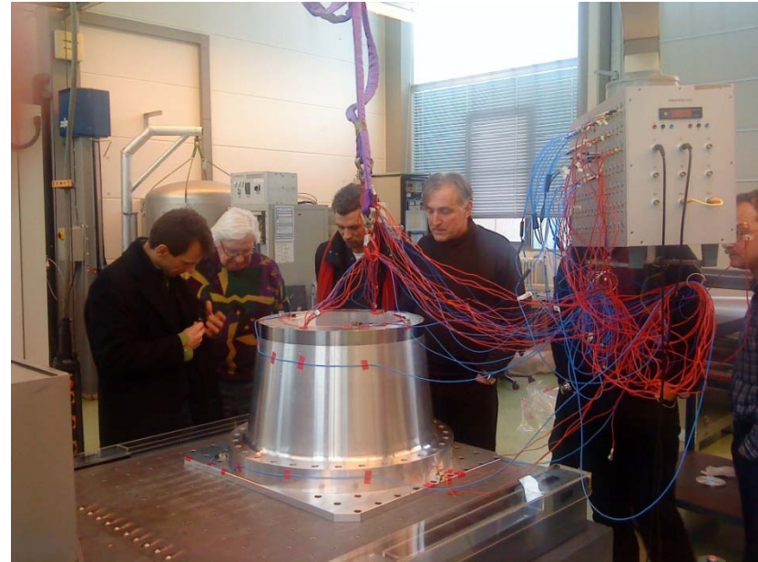
Mirror-EM on shaker at MPE
