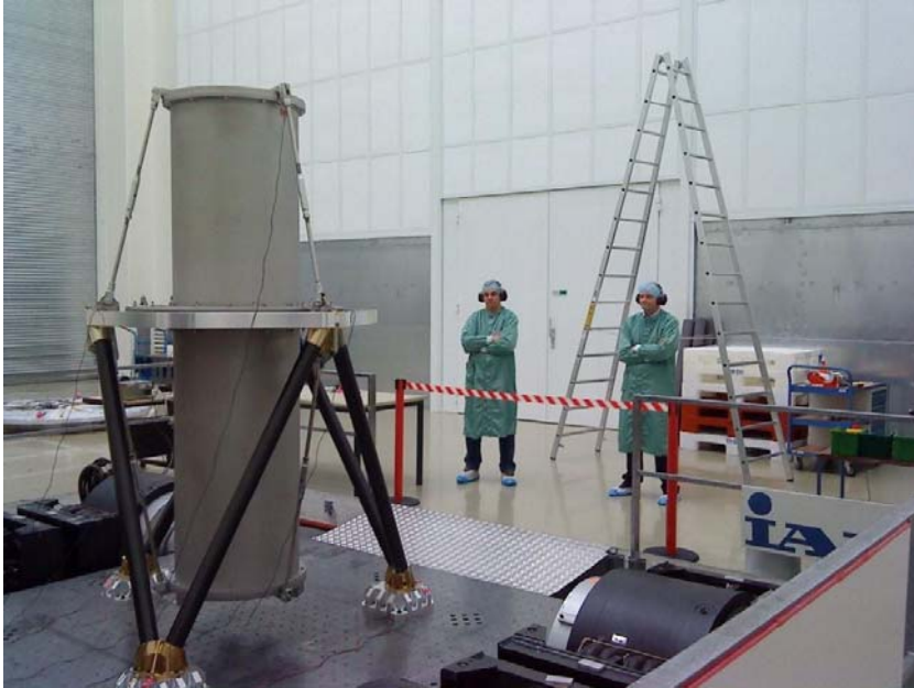
Structural Model on Shaker
