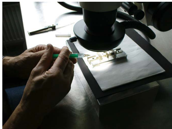
glue shrinkage tests
