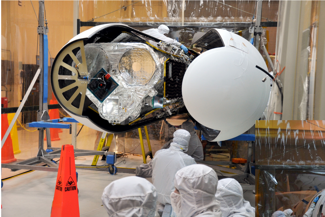
Fairing installation – March 2 nd
