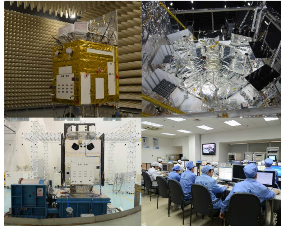
Electromagnetic compatibility test, thermal vacuum test, and mechanical test
