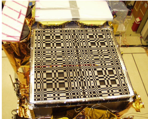
The IBIS coded mask , placed at 3.2m from detector. Built using 16mm thick W blocks, min.size 11.2mm
