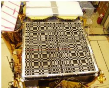
The IBIS coded mask , placed at 3.2m from detector. Built using 16mm thick W blocks, min.size 11.2mm
