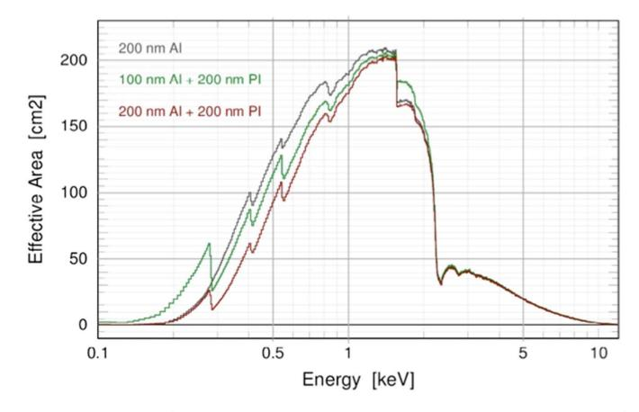
Effective areas of the three filter combinations for one eROSITA camera, composed of the expected effective area of one mirror assembly (averaged over the FoV), the filter transmissions, and the CCD quantum efficiency. All values are preliminary.
