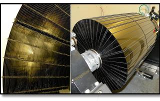
Conical Wolter-I approximation 133 shells (43 W/Si, 90 Pt/C)
