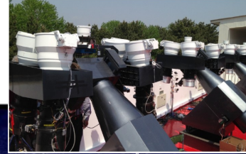
Ground Wide Angle Cameras 2 x 20 camera units \varnothing = 180 \text{ mm} // Total FOV ~ 5000 deg 2 500 – 800 nm Limiting mag ~ 16-17 (10 s)
