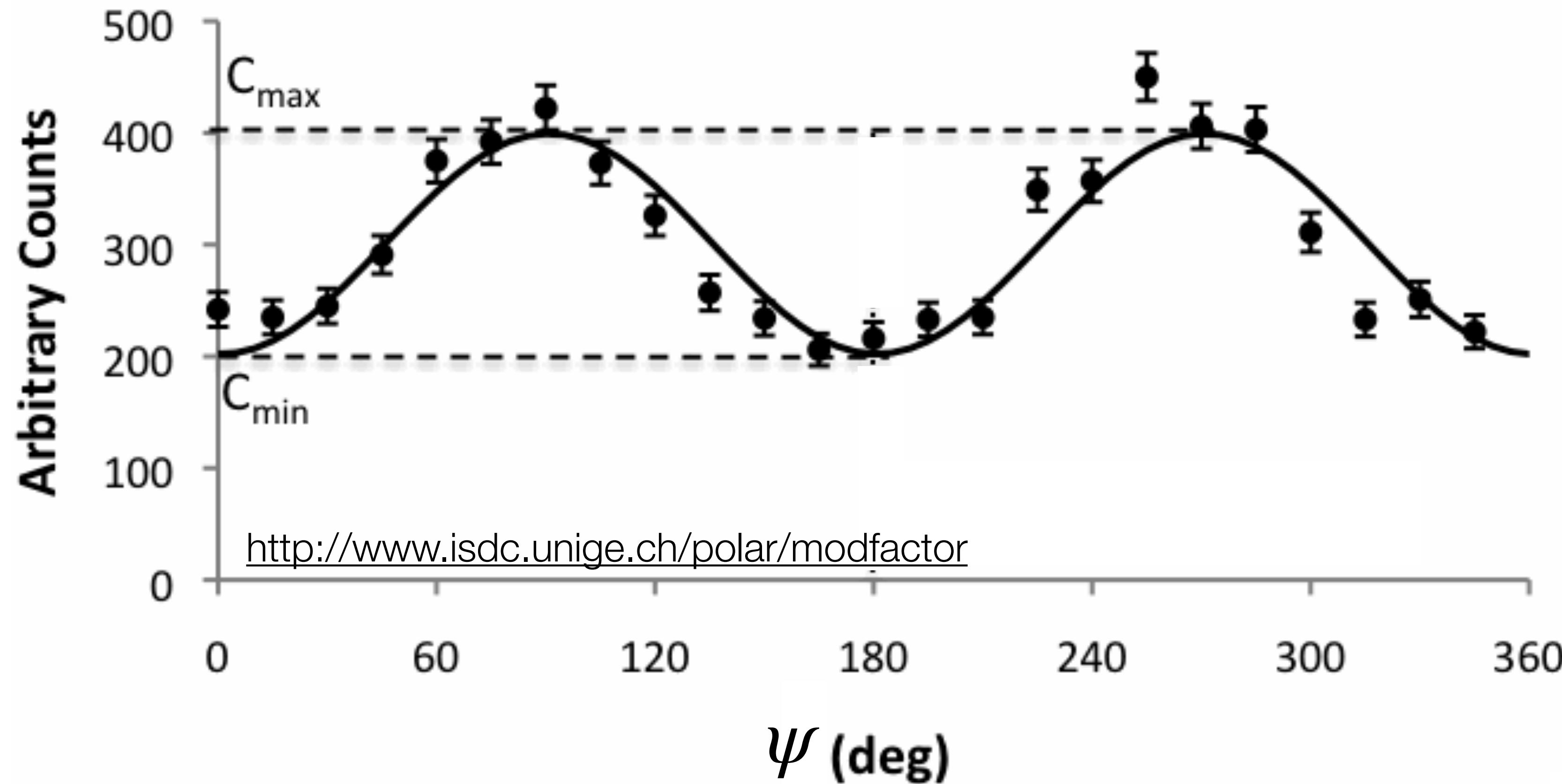
$$\text{Modulation Factor} = \mu = (C_{\max} - C_{\min}) / (C_{\max} + C_{\min})$$
