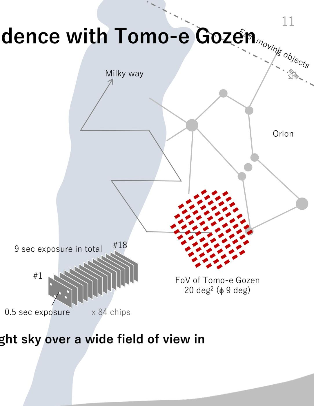
Video frames obtained with a single CMOS sensor, 2 frames/sec
