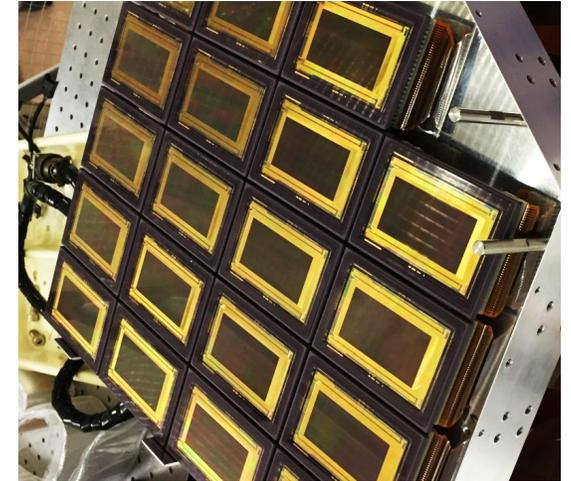
CMOS image sensors arranged along a spherical focal surface
