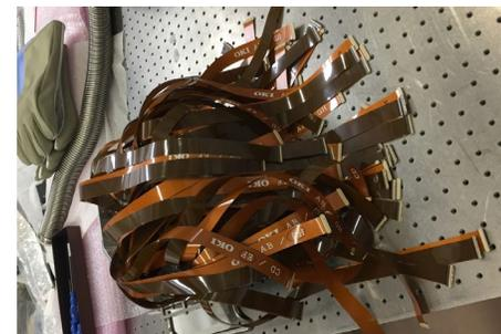
336 FPCs connected to 84 CMOS sensors
