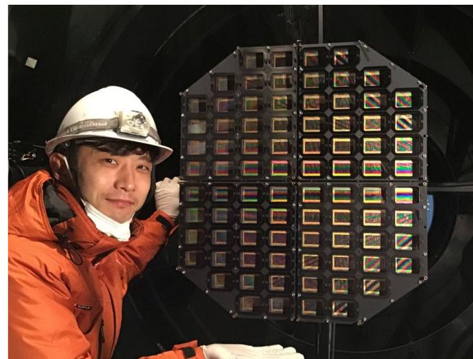
Tomo-e Gozen camera on the telescope's focal plane, features an array of 84 CMOS sensors.
