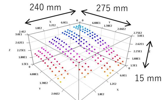
Top surface positions of the blocks measured precisely.
