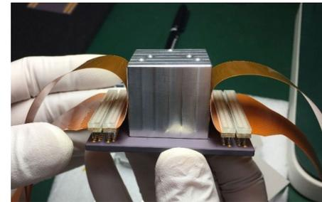
Blocks adhered to the back of each sensor
