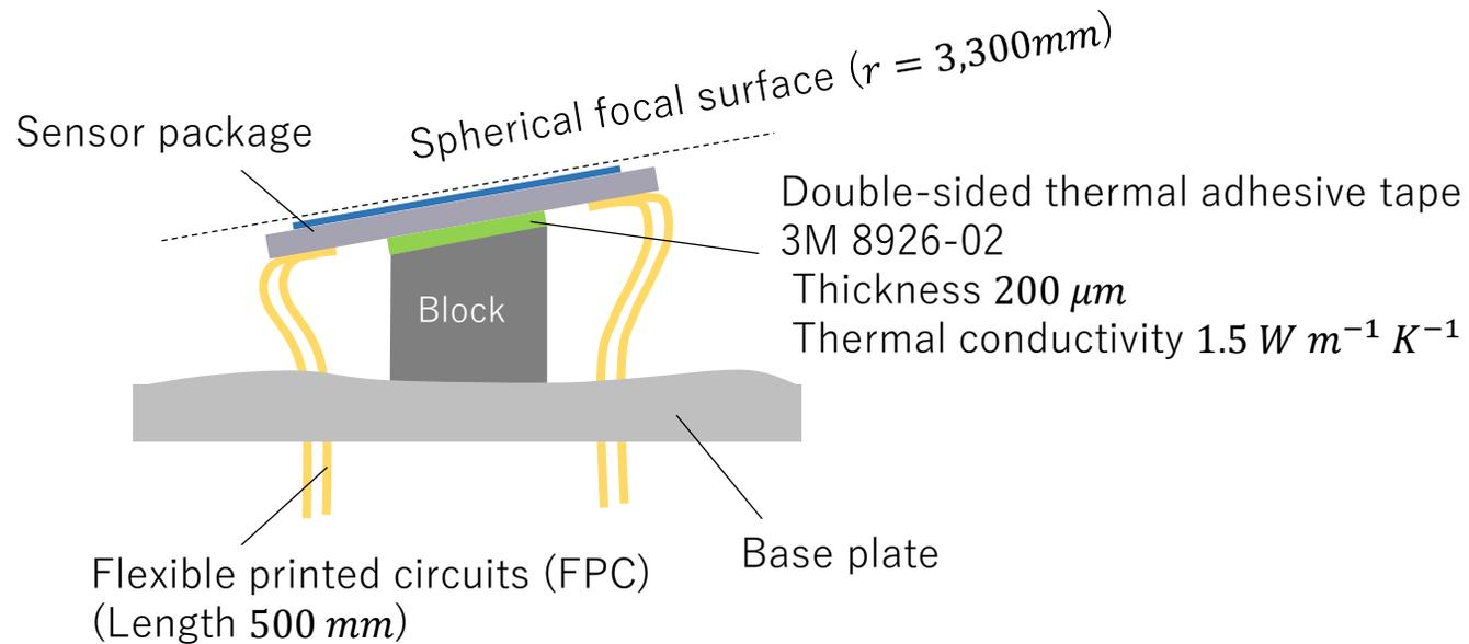
Achieved an alignment error of  $60\ \mu\text{m}$  peak-to-valley relative to the spherical focal surface.
